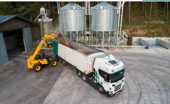
ippers were the first vehicles used by A.W. Jenkinson more than five decades ago and they remain an important part of the fleet. These roof-loaded, open-topped vehicles are mainly used for transporting bulk materials such as wood co-products to sites with restricted access. They use hydraulic rams to tip their loads out of the rear gate.
