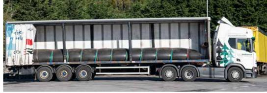
number of our standard curtain-sided trailers are fitted with a 18,000-litre collapsible neoprene tube designed to safely hold liquid-based resin. This product is used as a bonding agent in the manufacture of panelboard. On the return journey from the production site, the trailers have plenty of room to carry finished boards.
